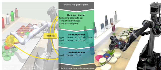
Fig. 1. Snapshot of a pizza domain task execution on the real robot alongside an illustrative description of the proposed framework.
