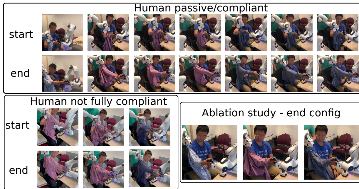
Fig. 15. Starting and/or end configurations for 3 different experiments: human passive/compliant, human not fully compliant, and the ablation study where the human remains static. For experiments where the human is not fully compliant, we also display with high transparency a nominal end configuration when the human is compliant. The deviation from the nominal end configuration is indicated by a blue arrow.
