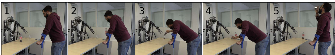
(a) Unassisted. REBA score during pouring and picking the glass varies between 4 and 5.
