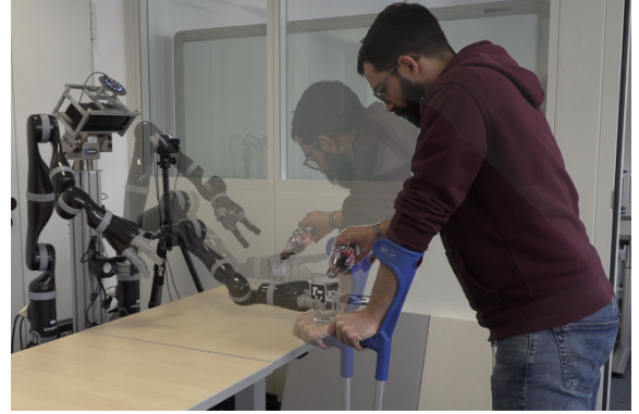
Fig. 1. Illustration of the presented concept in a supported pour-bottle-into-glass task. A robot intervenes to move the glass (transparent view) to a location on the table that enables an impaired user to comfortably pour the content of a bottle into it. The supported human (solid view) is enabled to perform the task optimally given an ergonomic metric. In the non-supported case, the (transparent) human needs to get into an uncomfortable posture.
