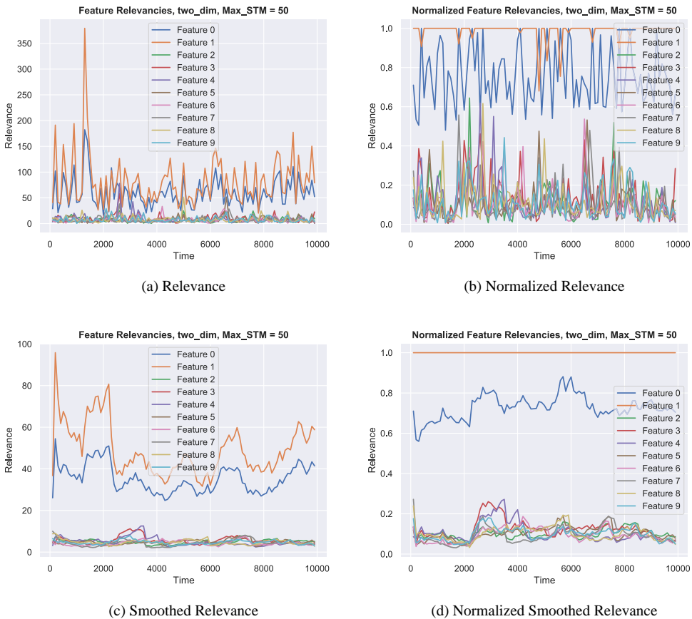
Figure 2. Different Relevance plots for the Two Relevant data set. (a) shows the relevance over time as computed by MLKR. (b) shows the same data as (a) but all values are normalized by the maximum value of each time step. (c) shows the relevance under a smoothed metric. (d) shows the same data as (c) but again normalized.
