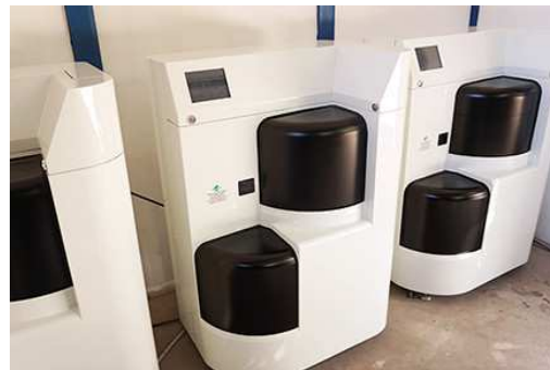
Figure 1: BSS (Honda Mobile Power Pack Exchanger) used in the pilot project 2
