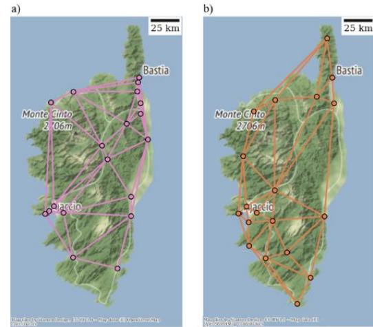
Fig. 5 UAM networks with 19 vertiports a) Heuristic Coverage Method (HCM) b) tradeoff solution of bi-level optimization F_k^* (AB-NDP).
