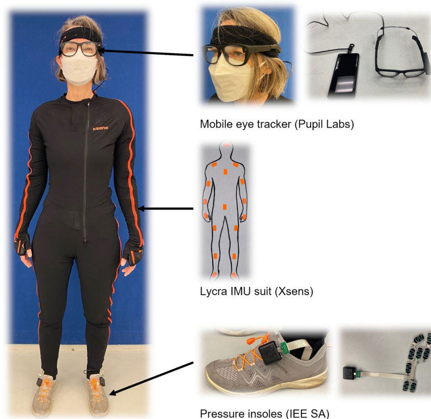
Fig. 4 The sensory equipment of the participants (left). They wore a mobile eye tracker, the Pupil Invisible Glasses 31 (top right), an Xsens full-body motion suit with 17 IMU sensors (middle right), and the IEE ActiSense Smart Footwear Sensor insoles (IEE S.A., Luxembourg) to record foot pressure data (bottom right). Note that the ICUs of the pressure insoles, the small black boxes attached to the shoes, also contain an IMU each. This means that there are two IMUs from different measurement systems attached to each foot: the IMU from the motion capture suit is located below the shoe tongue in the middle of the top of the instep and the pressure insole IMU is located on the shoe on the side of the top of the instep. The participant shown in this figure provided permission for their likeness to be used.
