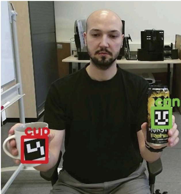
Figure 3. Clipped sample image of the object recognition visualization. The left marker is not tracked and therefore red. The right marker is currently tracked by the robot, which is indicated by a green bounding box. The learned label by the robot of each marker is written above the bounding boxes.
