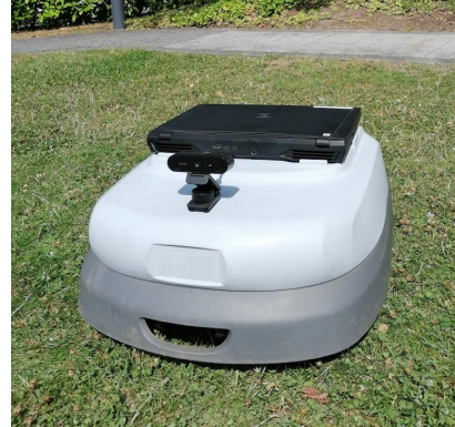
Fig. 1. Prototype robot. Research is demonstrated on a modified lawn mower robot with added camera and computational power. The system autonomously switches between mowing and following aesthetics gradients.
