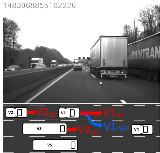
Fig. 3 Top: Screenshot of a Fast Successor scene. Bottom: Birds-eye-view representation of the traffic situation and the behavior options for the autonomous vehicle V1 and the relevant other traffic participants V2 and V3
