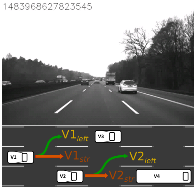
Fig. 2 Top: Screenshot of a Cut-In scene. Bottom: Birds-eye-view representation of the traffic situation and the behavior options for the autonomous vehicle V1 and the relevant other traffic participant V2
