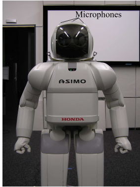
Fig. 2. Experiments are conducted on ASIMO whose legs, arms and head can move. Motion noise is recorded by an 8-ch microphone array with a circular layout embedded on ASIMO’s head.
