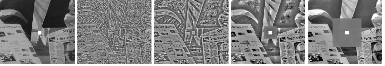
Figure 1. The left image shows the left Venus image altered by a rectangle of very high contrast. From second left to the right, mean and standard deviation normalized images are shown using filter sizes of 9x9, 21x21, 55x55, 149x149. Especially, for the larger filter sizes the suppression of the neighborhood of the high contrast rectangle is clearly observable.
