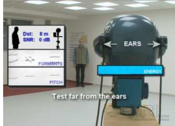
Fig. 4. Imitation in the parrot scenario. The system records human speech from several meters distance, extracts pitch and formants, and finally resynthesizes the speech using the extracted parameters.
