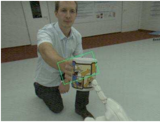
Fig. 5. Internal view of ASIMO when learning the relation between a speech label and the position of an object.
