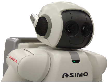
Fig. 1. HONDA's humanoid robot ASIMO modified to have human-inspired outer ears to improve sound processing.
