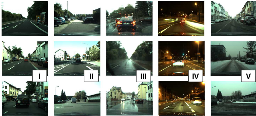
Fig. 13 Selected example images from streams I-V. All videos were taken in RGB color using a MatrixVision mvBlueFox camera at a resolution of 800x600. Used frame rates were 10Hz except for video II where a setting of 20Hz was used. Aperture was always set to 4.0 except for video IV where we used a value of 2.4. A self-implemented exposure control was used on both cameras, manipulating the gain and exposure settings of each camera.
