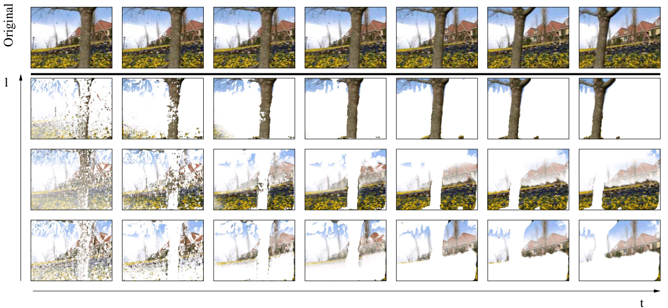
Fig. 6. “MPEG Flowergarden” sequence taken from a moving observer (top row). The different planes of the scene shift horizontally with different speeds depending on their depth: The tree moves fastest, the flower-bed at intermediate speed and the house and the sky background move very slowly. The system separates the overall measured motion into 3 layers of affine motion patterns, clearly segregating the different parts of the scene (bottom 3 rows).
