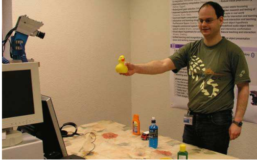
Fig. 7. The online learning scenario for recording training and testing images. Objects are shown freely by hand and a gaze control system using disparity focuses on the objects that are in the peripersonal space between user and the camera.
