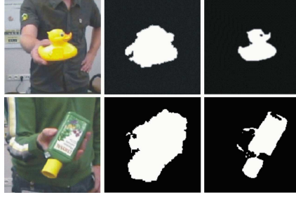
Fig. 1. A typical input image (left), the relevance hypothesis mask for the object (center), and the final ASDF object segmentation mask (right).
