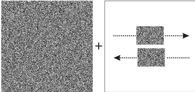
Fig. 2. Assembly of the first artificial motion sequence. The sequence is composed by a background pattern (left) superimposed with two patterns, simulating moving objects (right), that translate from left to right and vice versa.
