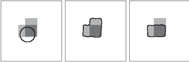
Fig. 7. Final level-set contour for region based level-set methods working on transparent motion. Left: Initial level-set contour for the gradient descent of Eq. 2. Middle: Assuming unimodally distributed data. Right: Using the pdf of the motion estimates instead of the velocity field and assuming multimodally distributed data.
