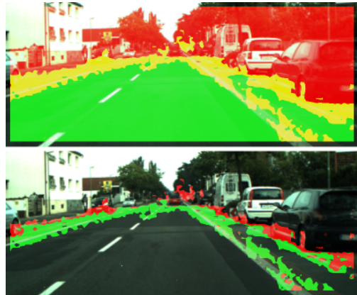
Fig. 5. Segmentation result in inner-city / overcast (frame 678). The upper image shows the distinct parts of the boundary region extraction: safe road (green), safe non-road (red) and the boundary region (yellow). In the lower image the segmentation result of the boundary detection is illustrated. The fused result gives a quality Q_I = 94,4\% ( th_{fus} = 0 ).
