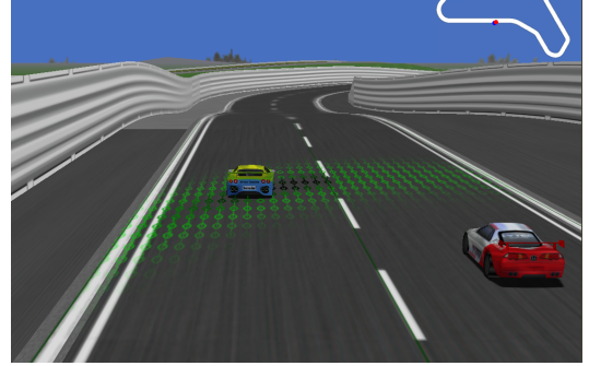
Fig. 3. A screenshot from the test scenario. The yellow car B is overtaking the red vehicle A , heading for the curve. The active grid nodes are drawn in perspective on the street.
