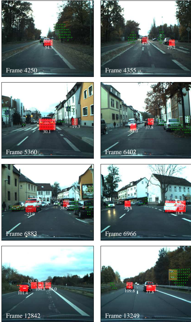
Fig. 3. Example images of the results, red points depict moving objects, green static ones. The moving objects show additionally rectangles of the temporal stabilization, where the color intensity indicates the certainty for moving. The average speed (km/h, after temporal stabilization) for the detected moving objects from our approach is also depicted. Note: in Frame 5360, the moving object on the right hand side is a bicyclist.
