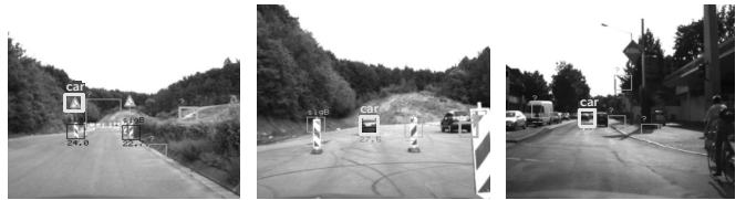
Fig. 3. Some performance examples of the FIRST system running on a prototype car. The left two images show operation in the construction site scenario it was envisioned for, the rightmost image shows operation in an inner-city scenario in Offenbach, Germany. Boxes in the images represent object detections, where the object identities are shown above the boxes. Possible object classes are “car”, “sigB” (signal board) and “?” (unknown object). Numbers below boxes show the distance to detected objects (if available) as measured by the radar sensor of the prototype car. In the leftmost image, the incorrect detection of a car is highlighted.
