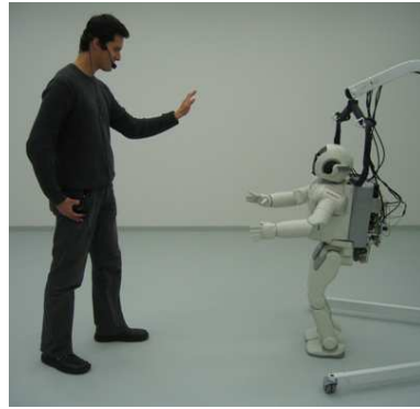
Figure 2: Experimental setup. The humanoid robot ASIMO interacts with a user in a reactive way by approaching and reaching for a proto-object. The user wears a headset for recording the speech signal. The user can teach the robot speech labels which describe behavior-relevant features of interaction: properties of proto-objects or the activity of the robot.
