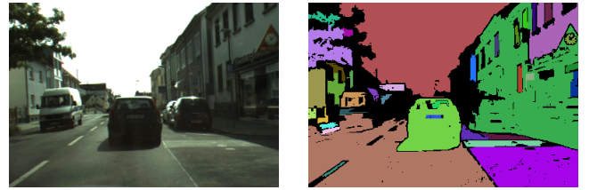
Fig. 3. The image on the right shows a false colored result of a simple Region Growing procedure applied on the left image. This preprocessing can be improved as there are some regions which cluster pixels from different planes, e.g. the car and its shadow are merged into one region. However, Region Growing already provides a sufficiently reliable starting point for the mapping of parameterizable surfaces.
