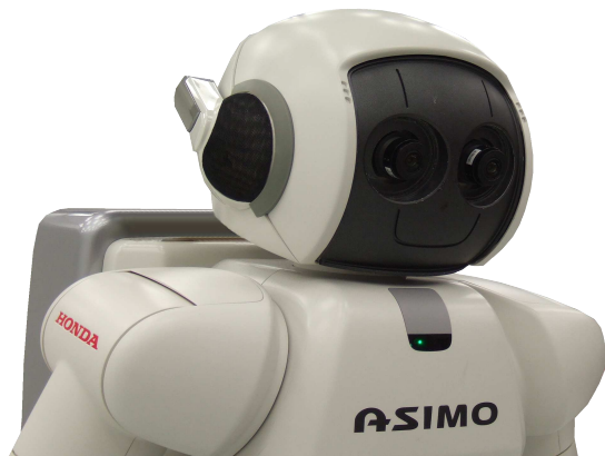
Fig. 3. Our humanoid robot ASIMO with custom-made, human-inspired ears.
