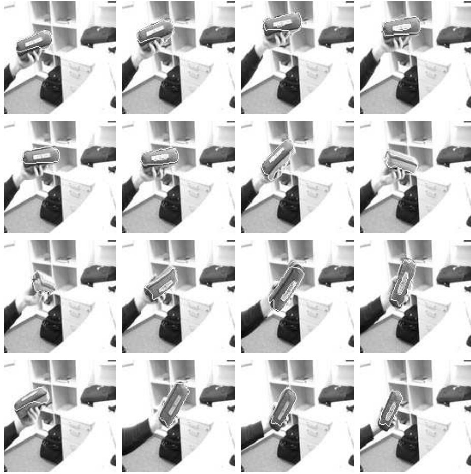
Fig. 6. In this case, the real world sequence is a moving pencil case. The pencil case is a non-rigid body, that translates, rotates and changes its scale but nevertheless is successfully tracked by the algorithm. This sequence was evaluated using the non-parameterized probabilistic model from Eq. 8.
