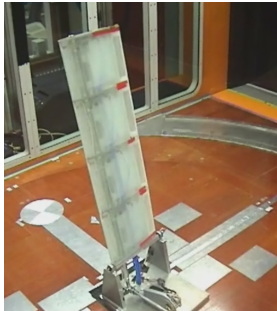
Figure 10: Adaptive Flapping Wing in Wind Tunnel
