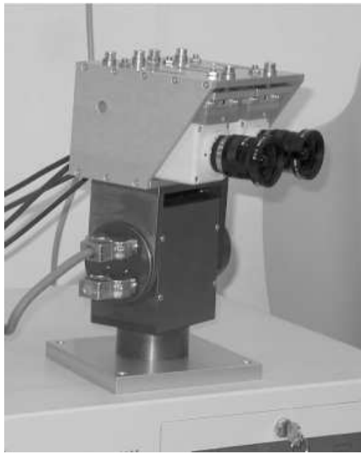
Figure 1. The stereo cameras on a pan-tilt head element.
