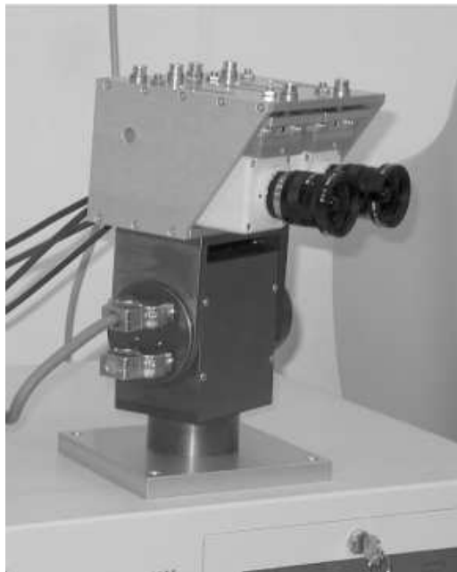
Figure 1. The stereo cameras on a pan-tilt head element.
