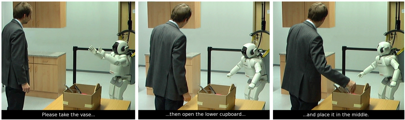
Fig. 1. Example of a multimodal three-chunk utterance delivered by the robot during interaction. Three different types of gesture are used (left to right): iconic gesture illustrating the shape of the vase; miming gesture conveying the act of opening the cupboard; deictic gesture pointing at designated position.
