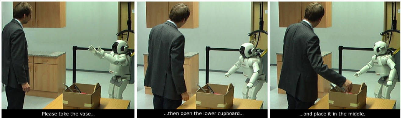
Fig. 12 Example of a multimodal three-chunk utterance delivered by the robot during interaction. Three different types of gesture are used (left to right): iconic gesture illustrating the shape of the vase;
